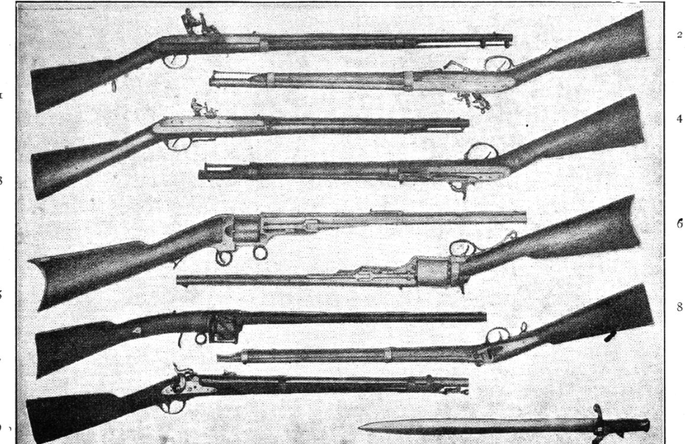
length of barrel 21 inches; calibre .54. The hook-shaped catch for the preceding pattern having not only proved inconvenient for the cavalryman but also capable of inflicting troublesome wounds, a remedy was sought in this device.
