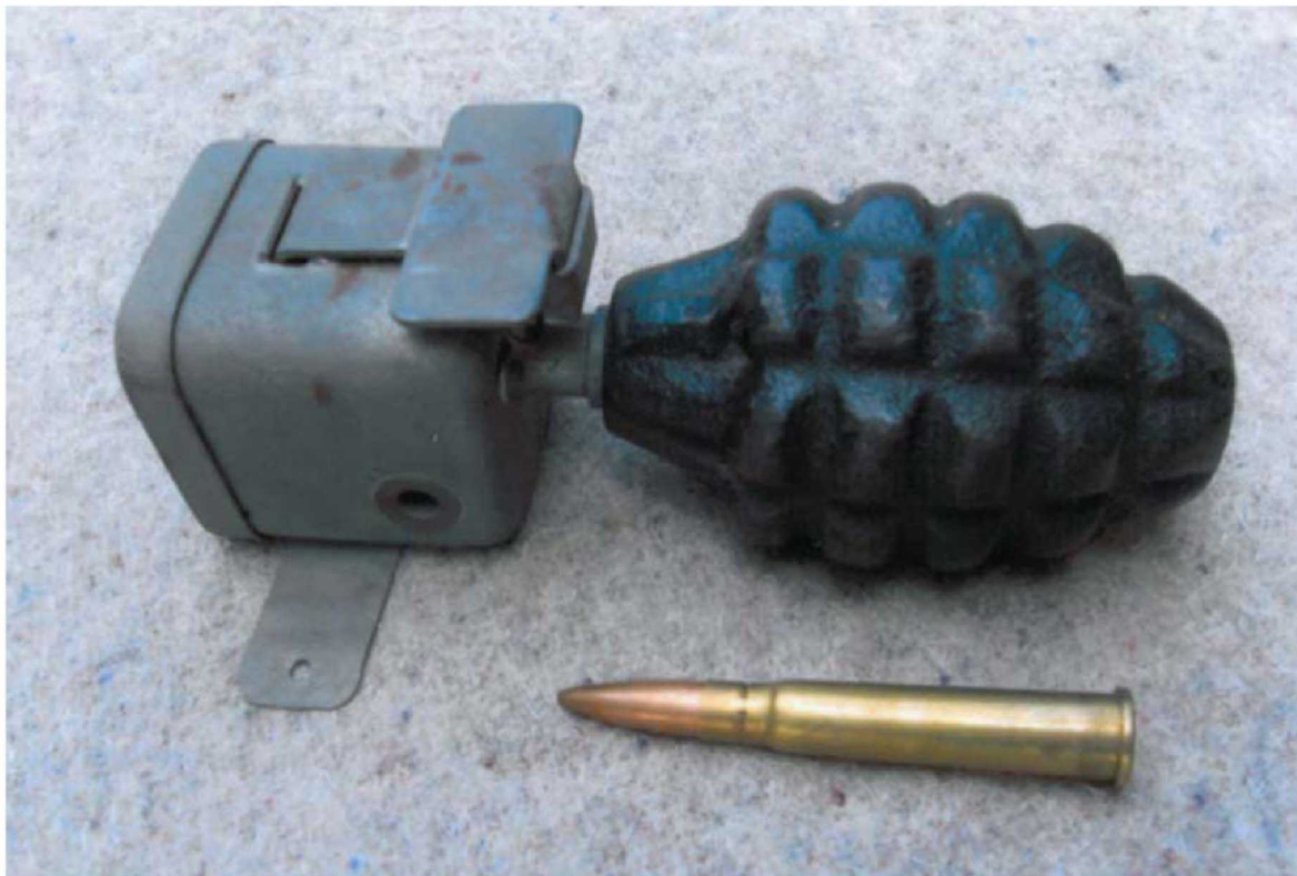
An M1 pressure-release firing device fitted to a US Mk II grenade; this required at least 2lb weight on the activation lever to prevent it from detonating. (David Gordon Collection)
