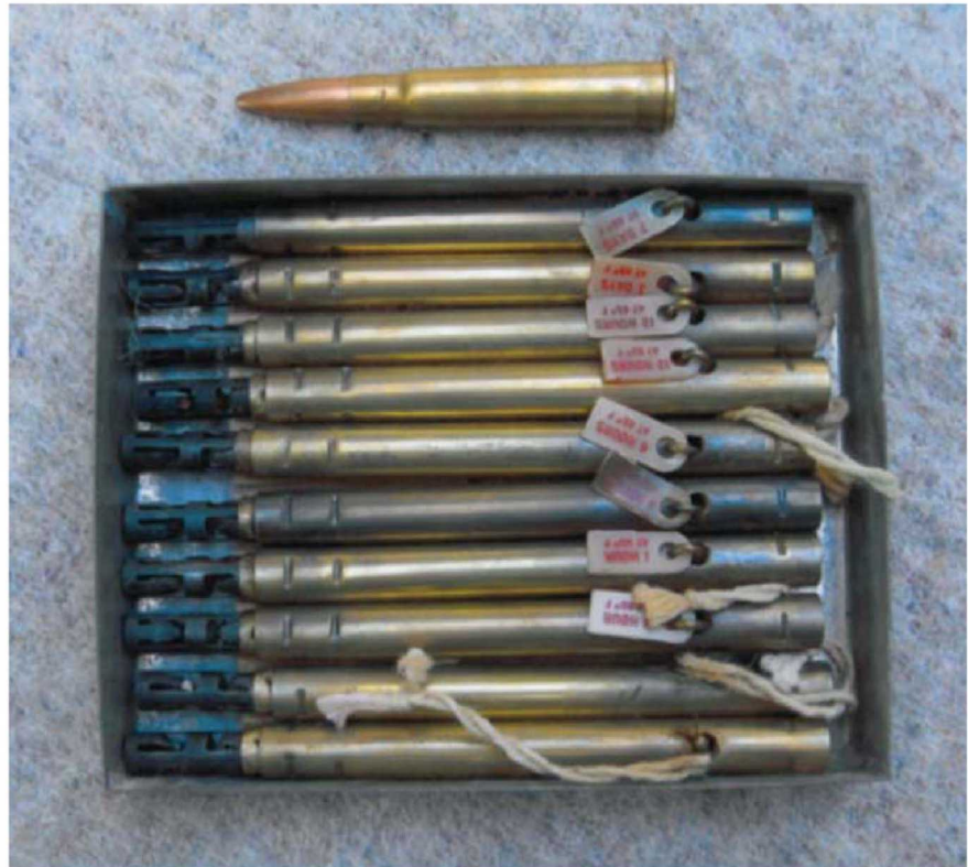
A carton of ten British No.9 Mk I time pencils ("L switches"). The safety pin included a white plastic tag with the delay time marked in red, ranging from minutes to days. (David Gordon Collection).
