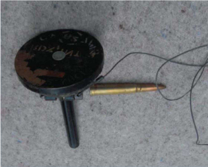
The British No.12 Mk I pressure-release switch was a 3in-diameter disc containing RDX/TNT. It was placed in a hole beneath a landmine, with the spike presumably resting on a solid base like a stone or piece of wood, and the disc flush with the bottom of the mine. A minimum of 2lb pressure was needed for safety. The arming pin was then pulled out with the cable, and the mine was camouflaged. (David Gordon Collection)
