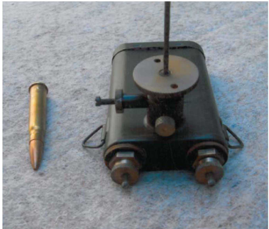
The British No.7 Mk I press/pull switch, later replaced by the No.13 Mk I. It could be activated by pressure on the round top plate or the rod extension, or by a pull-wire attached to one of the holes in the pressure plate. Compare with Plate B5 showing the earlier No.5 pressure-only switch. (David Gordon Collection)
