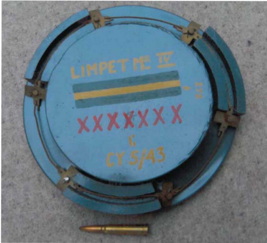
Bottom and top of a British Mk IV limpet mine; the magnets around its flat surface allowed it to be attached to ships' hulls, bridge girders, etc., under water. The other side shows a ring, by which the mine could be lowered below water level with the collapsible placement rod shown beside it. (David Gordon Collection)
